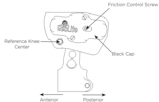
The suggested initial alignment is to position the reference knee center 3/8" (1 cm) in front of the Trochanter line. This is the most forward the socket should be at this time.
