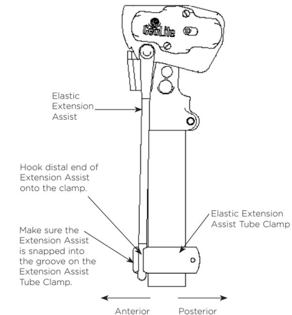
5. Position the Elastic Extension Assist Tube Clamp so that the arms of the Elastic Extension Assist are straight and not twisted, and so that there is equal tension in each of the arms, in order to prevent premature wear of the cover.
