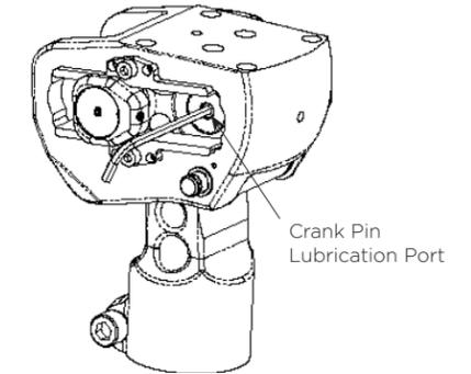
3. Place the tip of the pre-loaded Lubrication Syringe that was included with the knee (part no. 700-LU001) into the Lubrication Port. Push the plunger of the Syringe in about 20 mm. Try not to overfill the bearing chamber.
