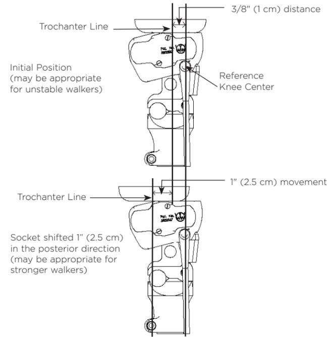
Keep the pylon and knee as vertical as possible in the anterior/posterior and medial/lateral planes to prevent uneven loading of the knee in the medial/lateral plane and difficulty initiating flexion in the anterior/posterior plane.
