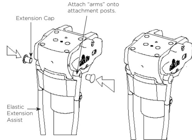
3. Using firm pressure, push each Extension Cap in until it snaps into position.
