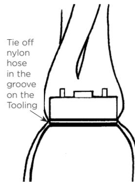
**Note: Do not allow the nylon hose to extend above the tie-off groove on the Lamination Tooling. Air leaks may occur in the finished socket if the nylon hose extends past the tie-off groove.**
