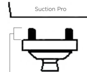
The length of exposed screw to engage with the Suction Pro must be between .4" (10 mm) and .6" (15 mm).
