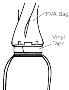
**Note: If the starting point of the tape is overlapped by more than 1" (25 mm), there may be air leaks in the finished socket.**
