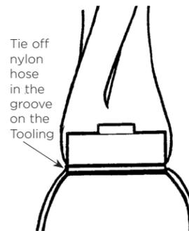
**Note: Do not allow the nylon hose to extend above the tie-off groove on the Thermoform Tooling. Air leaks may occur in the finished socket if the nylon hose extends past the tie-off groove.**
