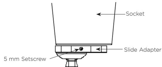
2. Connect a pyramid receiver component of your choice to the Slide Adapter. Tighten the setscrews using the torque and threadlocker specifications provided by the manufacturer of the pyramid receiver.
