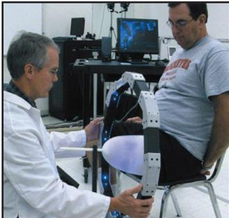
The OMEGA T-Ring is also a non-contact device, but instead of lasers and LEDs, it employs four synchronized optical imagers and four projectors mounted in a ring. The T-Ring projects lines onto a white sock that is worn over the patient's limb; the imagers "see" the lines and capture the three-dimensional shape.
