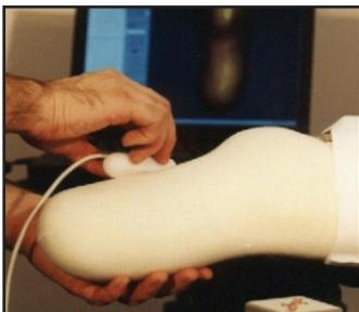
The third of the OMEGA devices, the Tracer Pen, is the only one that is not non-contact. A transmitter mounted on a tripod sends an electromagnetic signal that is picked up by the Tracer Pen and by a sensor that is strapped to the patient's limb. As the clinician moves the pen over the surface of the limb, a control unit determines the location of the Tracer Pen in space and conveys this information to the software.
