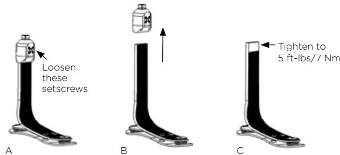
3. Apply Loctite 242 Removable Threadlocker (or equivalent) to the setscrews of the Torsion Receiver. Install the Torsion Receiver and tighten the setscrews to 5 ft-lbs/7 Nm (Figure C). Note: the shank must bottom out inside the Torsion Receiver.
